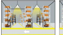
If there is no motion detected, the light will be remained at a low light level all the time.
