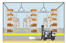
With sufficient ambient light, the light will not be switched on even if with motion signal.
