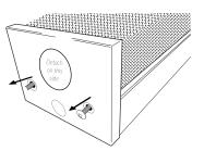
3. Slide out the diffuser from the end cap and completely detach it from the fixture.
