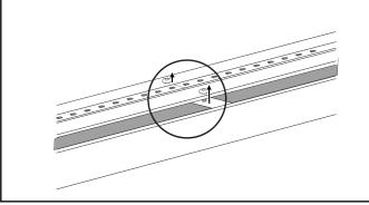
**5.** Gently remove the LED tray, ensuring proper safety measures such as using a lanyard or disconnecting the DC connector.
