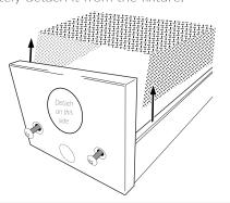
**4.** Proceed to loosen the two screws securing the LED tray.
