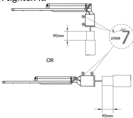
Pole diameter =  $\varnothing 60\text{mm}$
