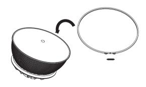
3. Then, secure both reflector and cover with the spring provided.
