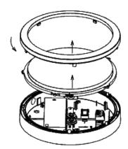
3. Separate the lamp compartment from the casing by disconnecting the connector.
