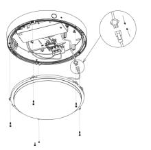
8. Rotate the bezel in clockwise direction.
