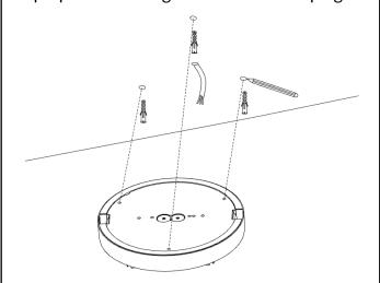
5. Pull cables through grommet. Fix the luminaire to ceiling with screws and washers provided.
