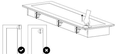
4. Lift one end of the luminaire into the cut-out hole and extend two crank brackets to latch to the ceiling while leaving enough clearance for the other end to connect main supply & DALI cable.
