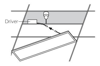
2. Remove or cut ceiling tile as dimension provided.
