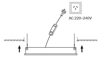
2. This luminaire is to be installed direct lay on T-Bar ceiling. For extra safety, this luminaire can be suspended from roof truss or concrete slab by using steel wires and hooked from the 4 hanging holes provided. (Steel wires not provided)
