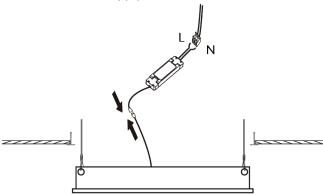
4. If the luminaire is installed with flex & plug, place the luminaire to the T-bar ceiling then insert plug to the appropriate supply socket.
