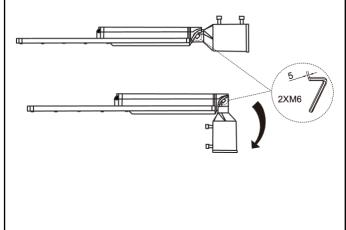
2. Loosen screw to open gear compartment cover.
