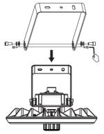
5. Drill at least 2 holes at wall and screw the trunnion arm to the wall.
