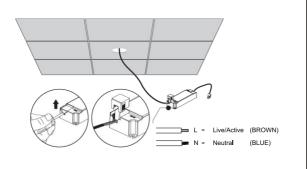
4. Connect driver's output cable to the downlight
