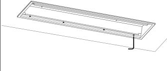
8. Close the frame. Screw the frame to the main body.
