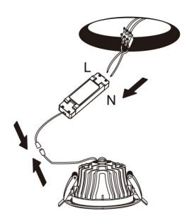
4. Fold up springs and fix downlight into cut out hole.
