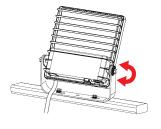
2. Mount the fitting to wall or ground and tighten the bolts using spanner.
