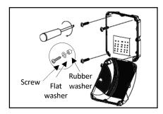
3. Connect cable Live (Brown), Neutral (Blue) and Earth (Yellow/Green) to the terminal block. Close cover and tighten all screws.
