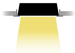
Plaster Recessed -with plaster frame
