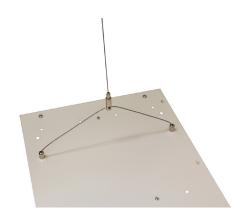
Secure the ceiling attachment to the ceiling or mounting surface using a 6 - 6.5mm screw/bolt. Where possible, screw directly into wooden beams, etc. If plastic wall anchors are to be used, choose the ridged type that flares out into the material
