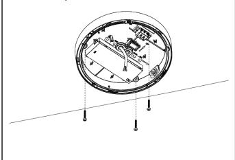
6. Connect the cables to terminal block accordingly. Then, fasten the cable with clamp. For luminaire with adjustable colour temperature, select a desired CCT.
