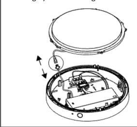
4. By using the casing as a template, mark and prepare mounting holes. Install wall plugs.
